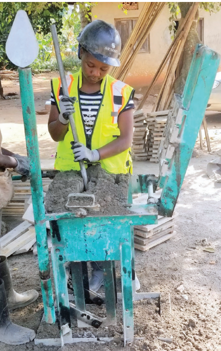
An apprentice operates the brick maker provided by Senders to give new skills
